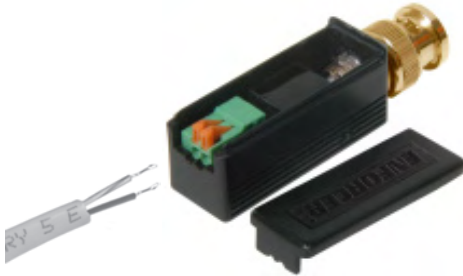
Figure 3: Inserting wires into video balun - use finger to pull back blades.
