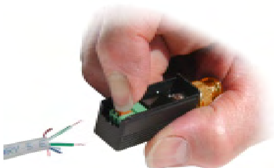
Figure 3: Inserting wires into video balun - use finger to pull back blades.
